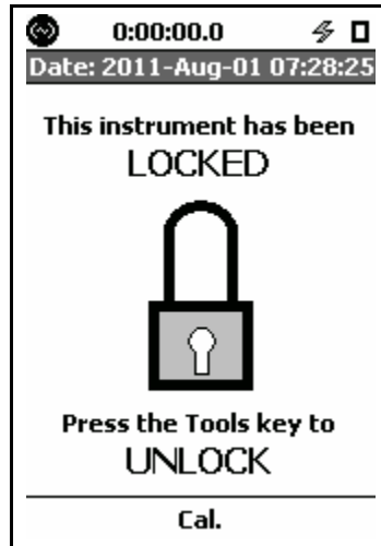
FIGURE 13-11 Locked with Calibration Permitted
